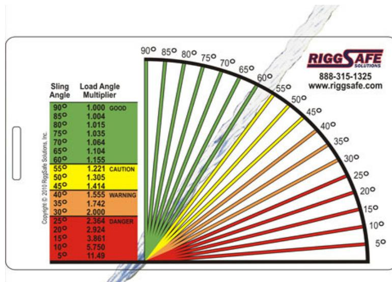
Rigging card. At 5deg the load ratio is 11.5x
